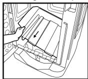
To aid cleaning, the liner tray can be removed to empty any debris that may have fallen out of the metal liner. Reservoirs in the liner tray can be easily emptied and wiped clean.
