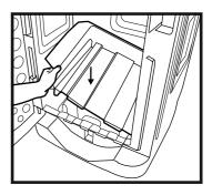
Reposition liner tray by pushing past the lugs so that it snaps into place.
