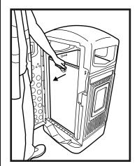
Remove liner by sliding out of bin.
