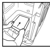
Insert bait box into position with the aperture facing the rear of the bin.
