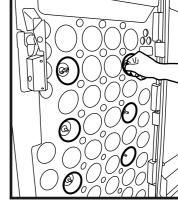
Place frame back into position and tighten wingnuts from inside the bin to secure.
