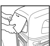
From outside the bin. pivot the panel forward from base then pull downwards to remove.
