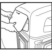
To insert a panel, position top bosses of the panel into holes in the body then push panel into position.
