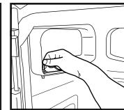
Using an M8 security allen key, replace washers and screws and tighten to secure.
