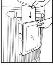
remove the frame and behind the clear panel.
