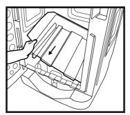
Remove the liner tray by pulling past lugs on bin body.
