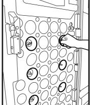
Remove all six wingnuts and washers from the unscrewina anticlockwise.
